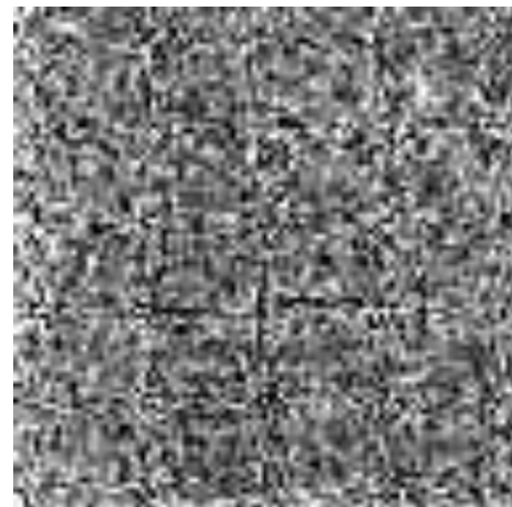
Figure 5: Example of non-uniform noise texture due to spatial interpolation processing. The contrast has been enhanced here.
