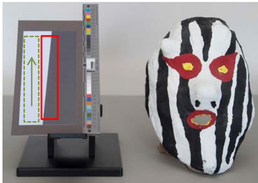
Test image for resolution and illumination evaluation, and. effective illumination profile
